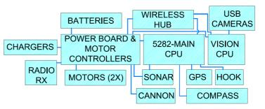
Figure 3: ASV subsystems block diagram
